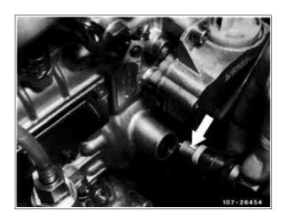
Connect position sensor according to connection diagram.
