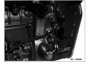
2 Turn position sensor into the governor housing. Ensure that the guide pin of the position sensor (arrow) faces up. Tighten union nut by hand.
